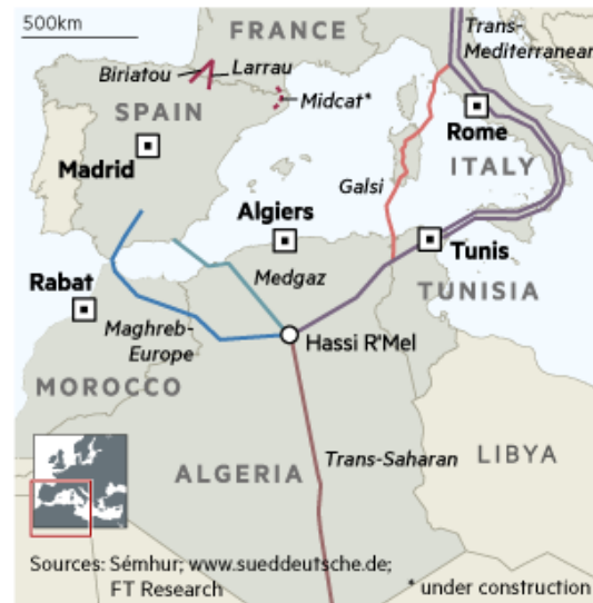
Gas pipelines from Algeria to Europe
